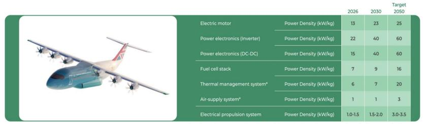
\*For thermal management system and air supply system the power used to calculate power density refers to amount of heat dissipated, and compression power required to support the system.
