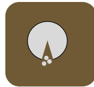
Active Material Cracking
