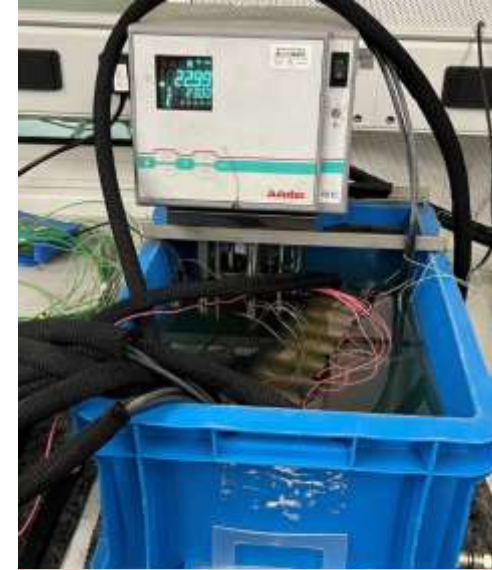
MoliceL P45B Cell Ageing Rig
